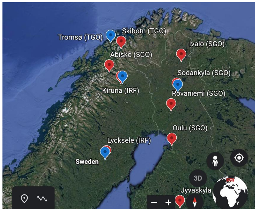
Figure 4.2 Sites of ionospheric measurements in the north. Red markers indicate riometers, and blue markers indicate ionosondes. The sites are run by Tromsø Geophysical Observatory (TGO), Swedish Institute of Space Physics (IRF) and Sodankylä Geophysical Observatory (SGO).
