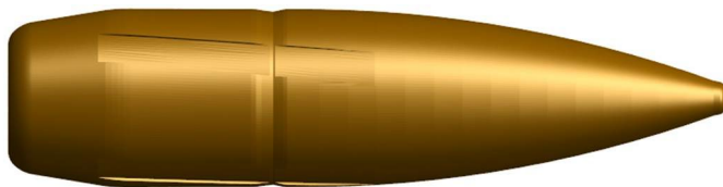
Figure A.1 Model of the 7.62 mm NM258 projectile. The geometry (except the rifles) is based on measurements of an unfired specimen. The depth of the rifles was measured on a specimen that was fired from an HK417 rifle.
